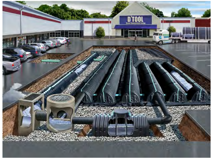
Permeable Paving and Gray Water Capture, Retention, and Park Irrigation System.
