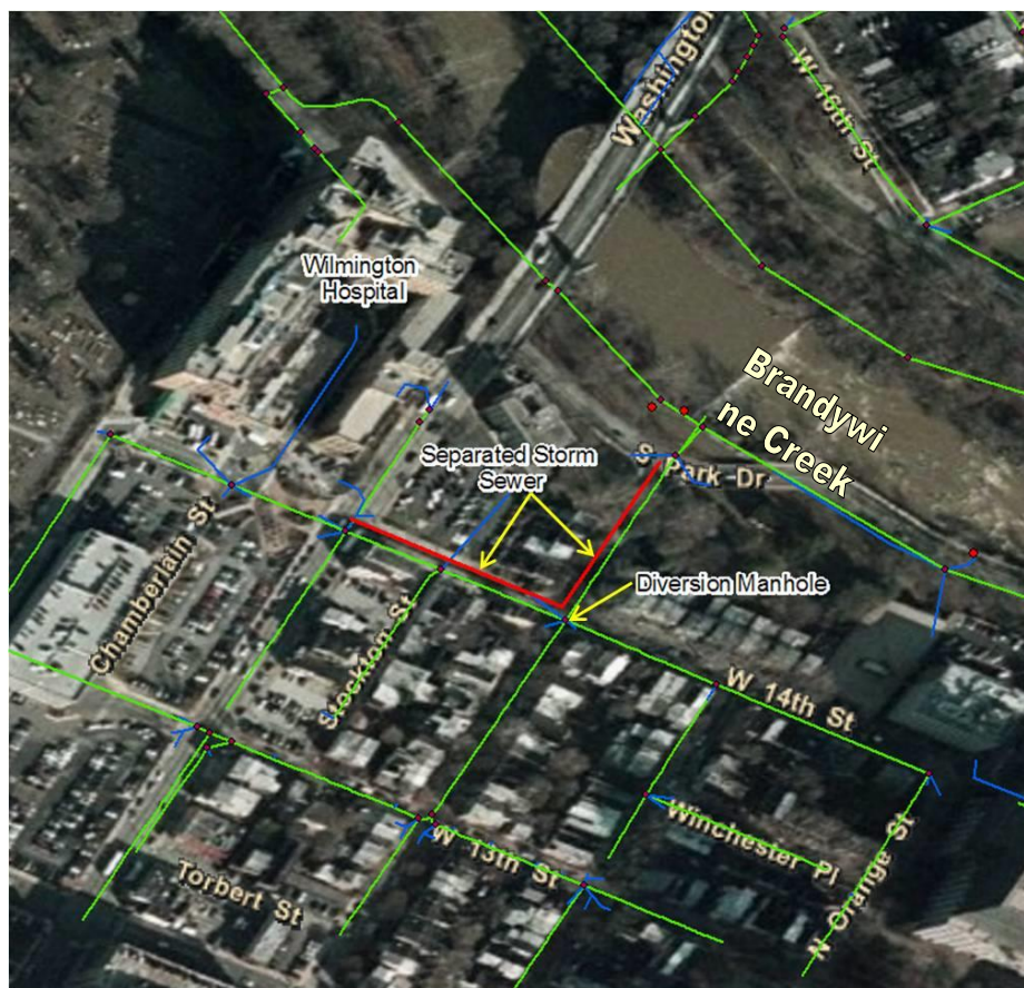
FIGURE 9: WILMINGTON HOSPITAL SEWER SEPARATION PROJECT
