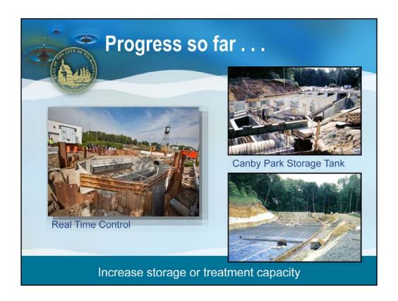
The City has already invested nearly 30 million in capital projects to achieve compliance with Combined Sewer Overflow regulations. This was achieved using traditional infrastructure improvements such as sewer separation, WWTP upgrades, an underground storage tank in Canby Park with a capacity of 2.7 million gallons, and Real-time Control – which optimizes in-system storage using predicted and actual rainfall data/ Optimized system O&M.
