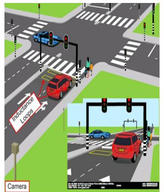
The second digital image will show the violating vehicle beyond the violation point proceeding through the intersection, the red signal phase, in addition to data about the violation that appears at the bottom of the image.
